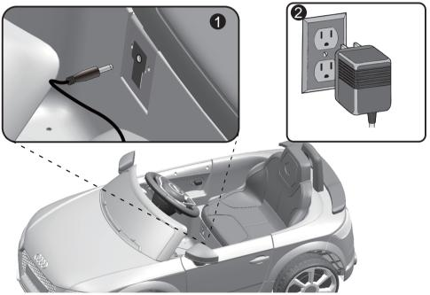
1. Plug the charger port into the input socket. (the socket is below the seat) HINT: If your vehicle equipped with the Multi-function Dash, the Charging Socket is on the dash, please see page 15 <Use the Multi-function Dash> 2. Plug the charger plug into a wall outlet. The battery will begin charging.
