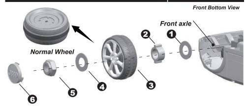
Remove all the parts from the front axle.
