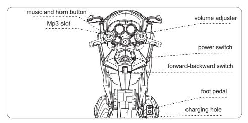
power switch, forward/backward switch are on the tank, pedal switch is on the right.
